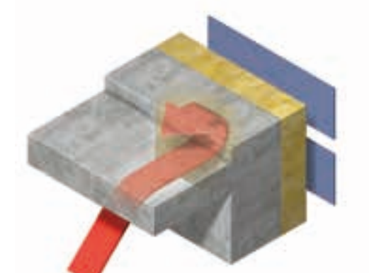
Minimisation of thermal bridging
